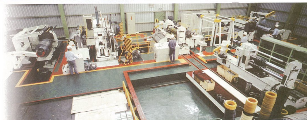
各式五金捲片及 表面處理鋼材之分條設備 Slitting line for various metal coil and steel coil of surface be treated.
