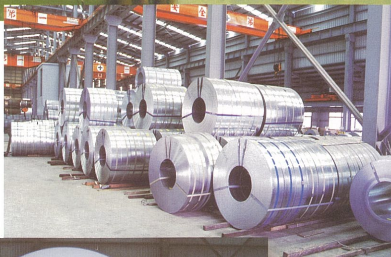
高張力捲取之卷帶成品 Coil products by high tension recoiling
