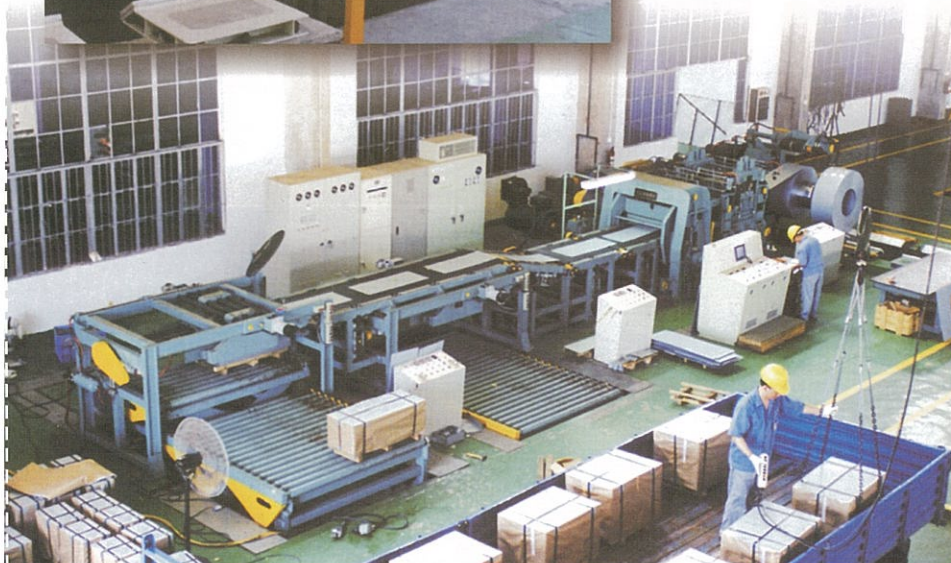
小型飛剪設備 切片厚度0.2以上 Mini cut-to-length line of rotary shear type Cutting thickness:0.2mm up
