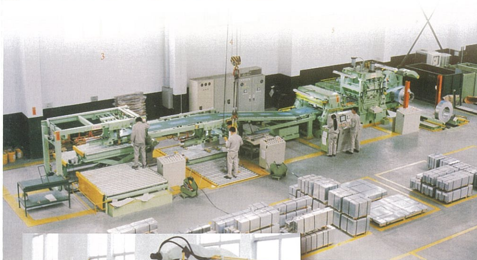
小型飛剪設備 切片厚度0.2以上 Mini cut-to-length line of rotary shear type Cutting thickness:0.2mm up
