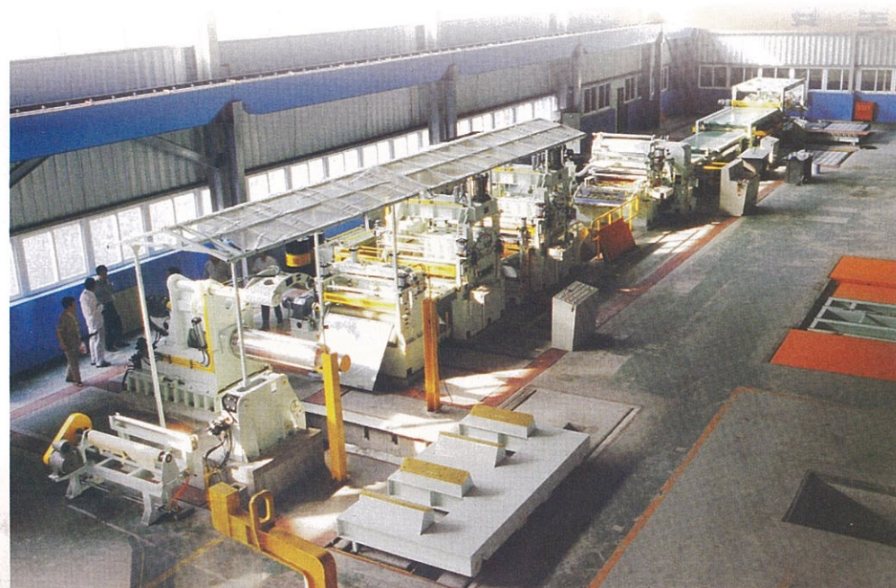
6-Hi 精整機附快速上升 6-Hi precision leveller with quick-lifting
