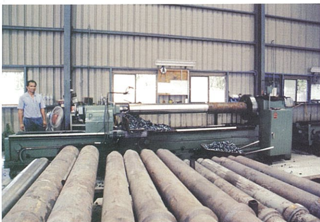
分條刀軸毛胚 Rough turning for slitter shaft
