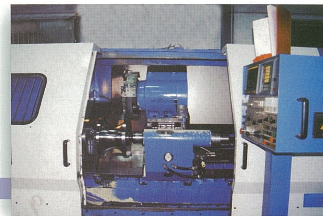
製管滾輪熱處理後之NC自動精車 Precision turning by NC-lathe for forming roll after hardening
