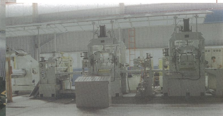
雙精整機一部 4HI一部 6HI以輪替對SUS-BA.2B或EG之整平 Twin precision leveller, one of 4-Hi, the other of 6-Hi could be substituted for levelling of SUS-BA. 2B or EG.
